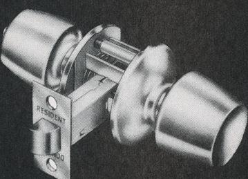
**Operates by knobs from either side except when outside knob is locked by push button on inside knob. When so locked, no means of entrance is provided. Inside knob in operation at all times. Lock is automatically released by turning inside knob or depressing latch bolt.**
