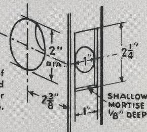
Requires drilling of two holes only and slight mortising for lock front and strike.
