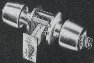
**Push Button locks outside knob. Lock opened by key in outside knob or by turning inside knob when outside is locked.**
