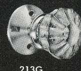
Locked by moving slide on inside rose; has automatic kick-off in case set is automatically locked with door open. Emergency key operates through opening in outside rose.
