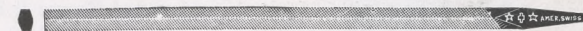
Locksmiths' File This file is designed especially for locksmiths for duplicating and dressing down cylinder keys. It is 7" long and has two cutting sides. The angle is 100°, which is just right for general duplicating.
