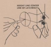
MARK FOR LATCH HOLE ON HEIGHT LINE. MARK HOLE IN CENTER OF DOOR THICKNESS FOR 13" TO 13" DOORS. FOR DOORS OVER 13", WHICH REQUIRE SPECIAL LOCKS, MARK HOLE 34" FROM OUTSIDE FACE OF DOOR
